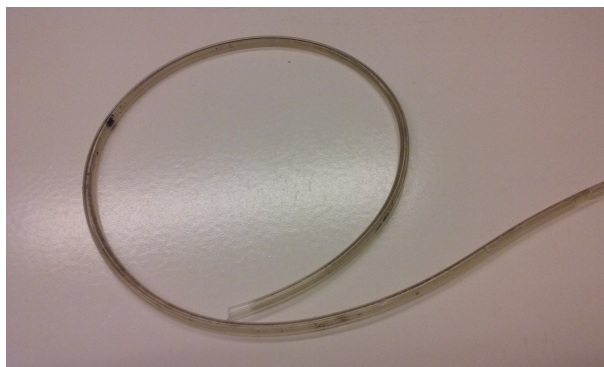
Figure A.6: Microfluidic tube after polymerisation of dopamine.
