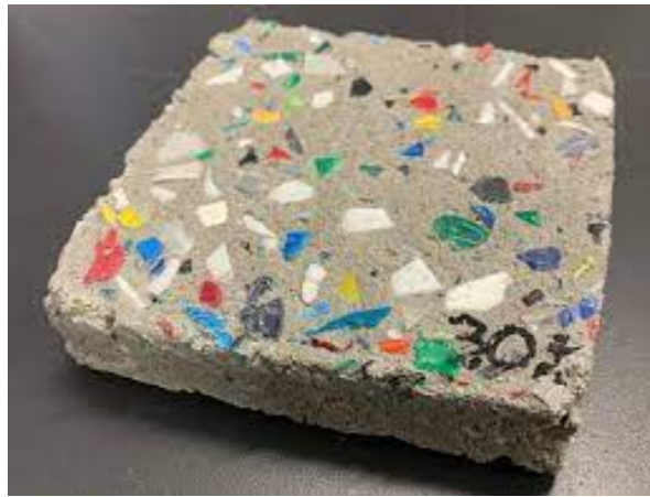
Figure 2.1: Concrete block containing recycled plastic bottles [24].
