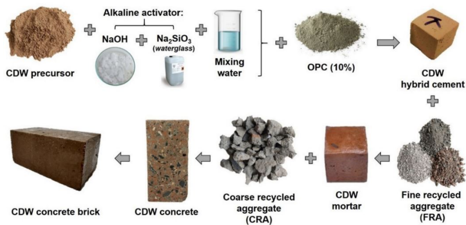
Figure 2.2: Recycling process of crushed sand into concrete blocks [23].
