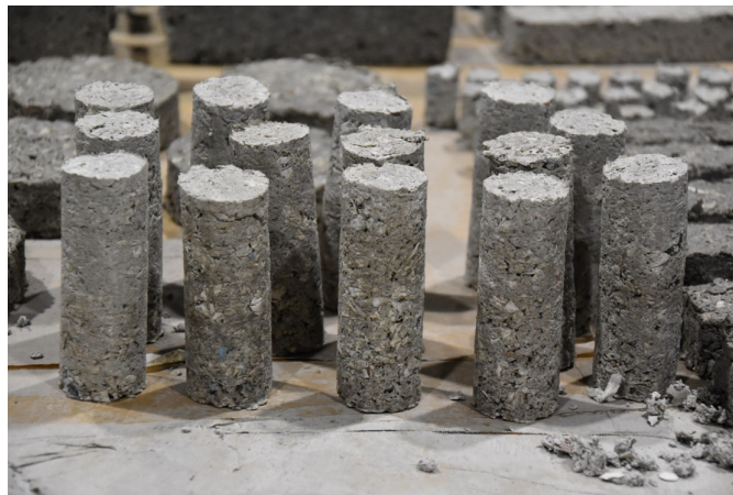
Figure 3.18: Example of samples that are sent to the tomograph (picture taken by Mélanie).
