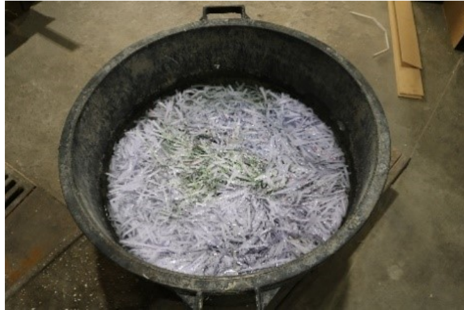
Figure 3.3: Soaking of paper in water basin (picture taken by Mélanie).
