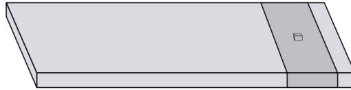
Figure 3.5: Step ②: Adhesive tape on PDMS.
