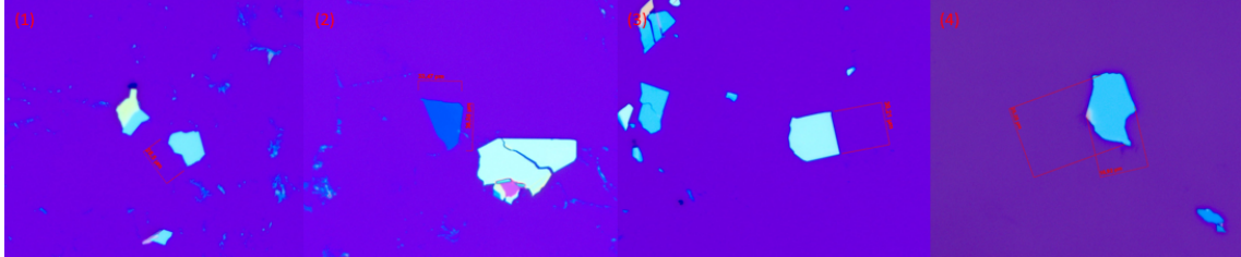
Figure 4.4: Microscope images of 4 selected h-BN flakes of different thicknesses. Despite defects and impurities, all of them were kept for transfer as their surfaces remain flat.
