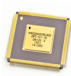
Figure 1.10: The digital programmable controller ASIC in its CQFP package. Courtesy of [15]
