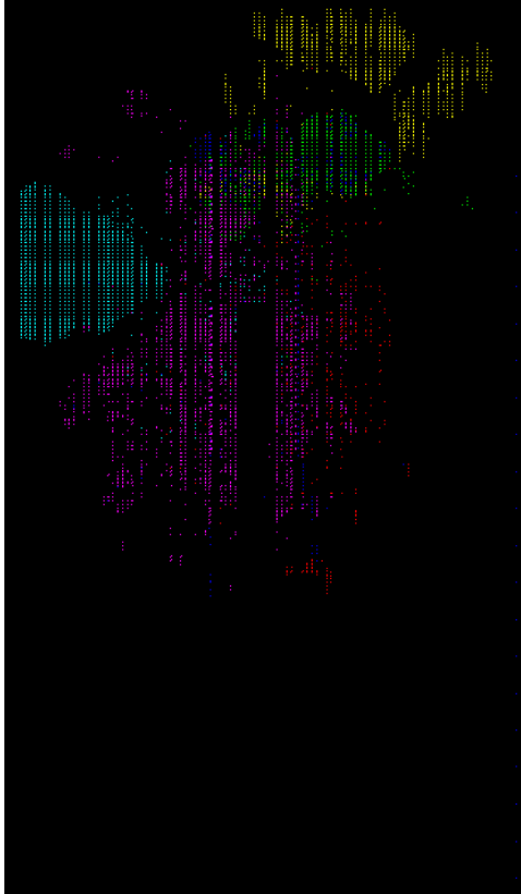
Figure 4.5: 5 radix bits. Magenta = Memory controller, Cyan = Blake2b, Green = collision, Yellow = Radix, Red = UART
