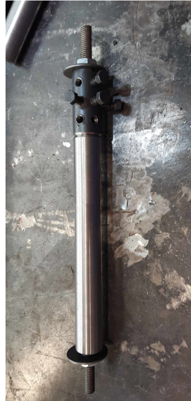
Figure B.11: Centered coupler before welding
