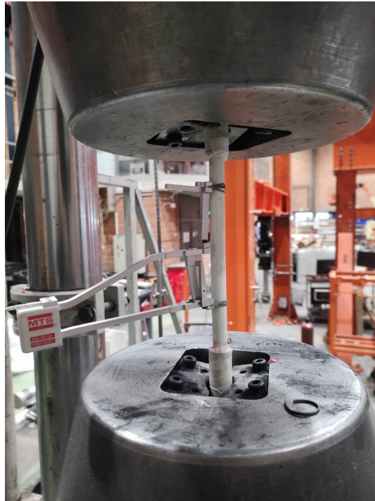
Figure 3.12: Monotonic test setup of the IRT-M2P bars with small aluminium anchorages and a 100mm extensometer
