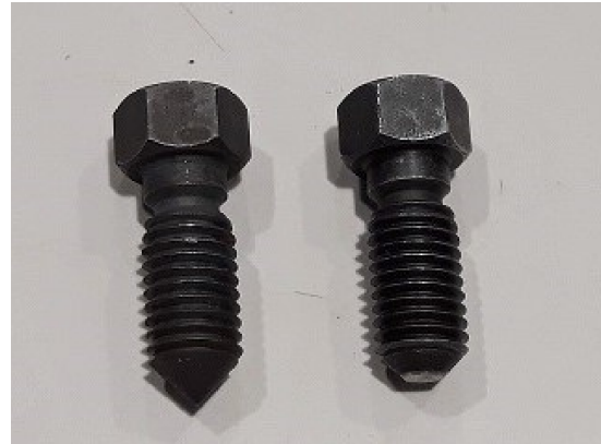
Figure 2.10: Difference between a normal screw and a flattened-head screw. From Herzezel et al.[35]
