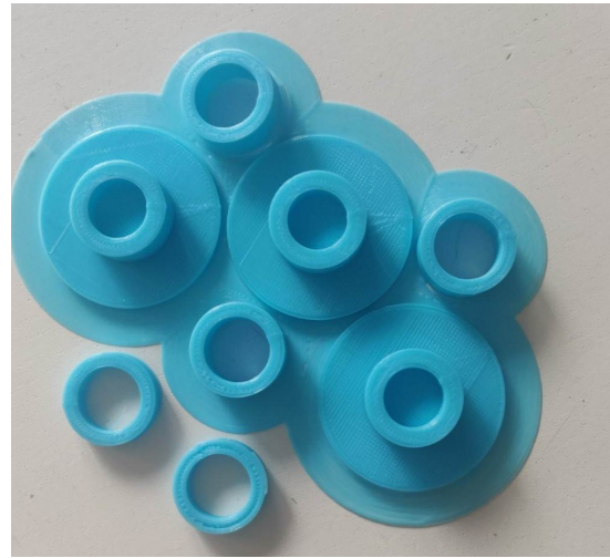
Figure B.13: 3D printed rings for the centering of the GFRP
