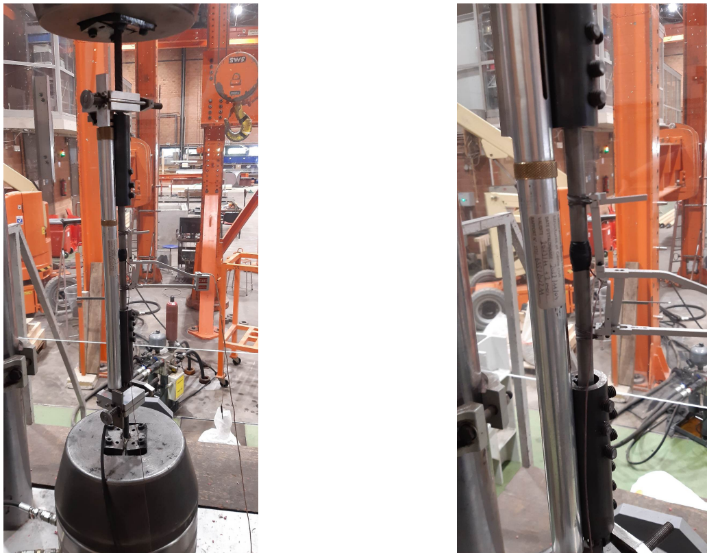
Figure 4.8: Test setup of the SMA-Steel configuration as in Fig4.7, with two extensometers and a thermocouple on the SMA (right)
