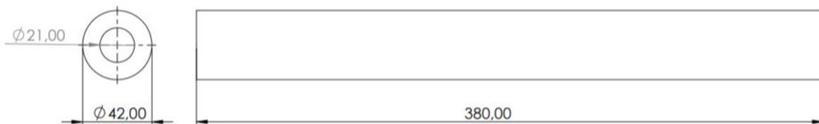
Figure 3.5: Anchorages dimensions for 13mm GFRP rebar
