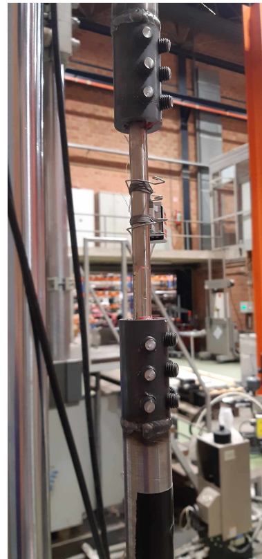
Figure 4.34: Slippage of the SMA during the GFRP-SMA cyclic test
