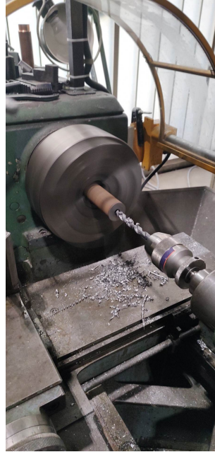
Figure B.2: Drilling with the metal lathe
