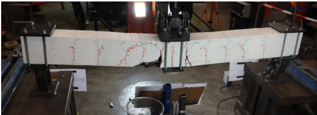
Figure 5.26: Cracks repartition on N1 steel beam[46]
