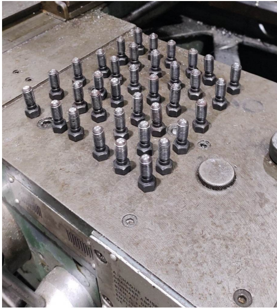
Figure B.12: Flattened screws, provided with the sleeves
