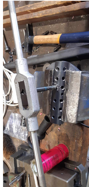
Figure B.7: Tapping the holes
