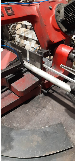
Figure B.1: Cutting of the steel tube
