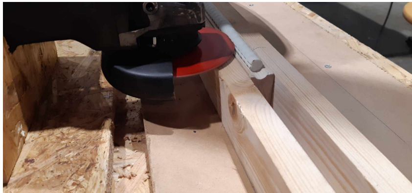
Figure 4.26: Grooving of the GFRP bar
