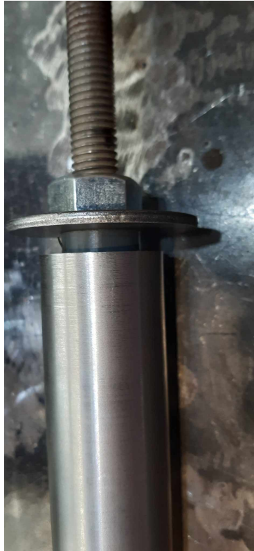
Figure B.10: Centering of the GFRP part with 3D-printed rings
