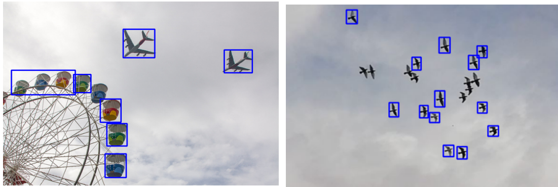
Figure 4.15: Left: Detection with the ResNet50 model trained without the non-bird dataset. The model trained with it, doesn't detect anything. Right: Detection with the ResNet50 model trained with the non-bird dataset. The detection without it, is shown in Figure 4.13.
