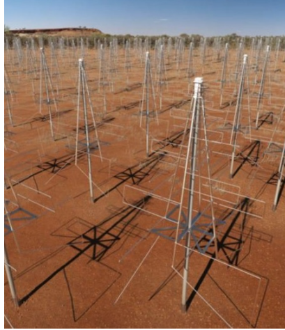
Figure 1.4: Artist's image of SKA-low array dipole antennas – Swinburne Astronomy Productions/ICRAR/U. Cambridge/ASTRON. Reference: [1].
