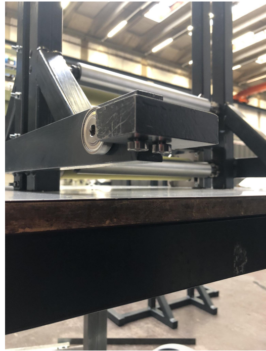
(b) Bearings of the railway cart
