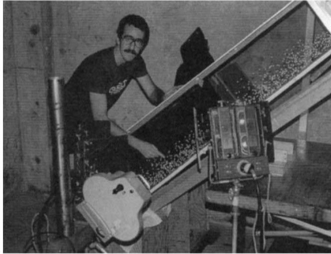
Figure 1.2: Drake performing his experiments in 1991 with an experimental chute, measuring 3.7 m in length, 0.5 m in depth, and 6.7 mm in width, where a typical dispersal flow occurs. Plastic spheres with a diameter of 6 mm are fed from a hopper located above and behind the upper end of the chute. A high-speed camera, operating at approximately 1440 frames per second, captures particle motion. From [22]
