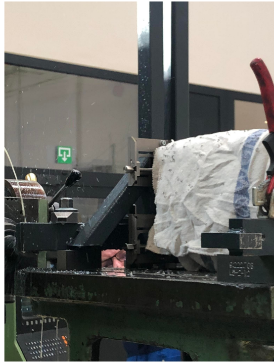
(b) Roller protection for chip expulsion
