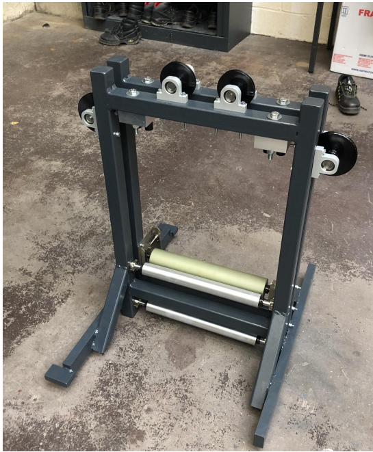
(a) The railway cart fully assembled
