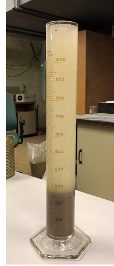
Figure 8.12: Computing initial volume fraction
