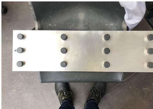
(c) Plate (26) with its 12 dampers
