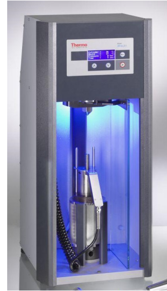
Figure 2.9 Injection molding machine of the lab : Thermo Scientific TM HAAKE MiniJet Pro .
