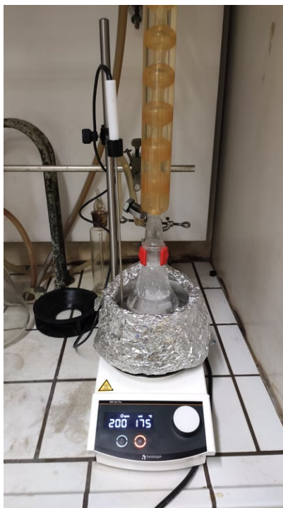
Figure 4.3 Depolymerisation setup with a condensation setup to keep the volatile reactant in the nitrogen gas and a system of water condensation mixture.
