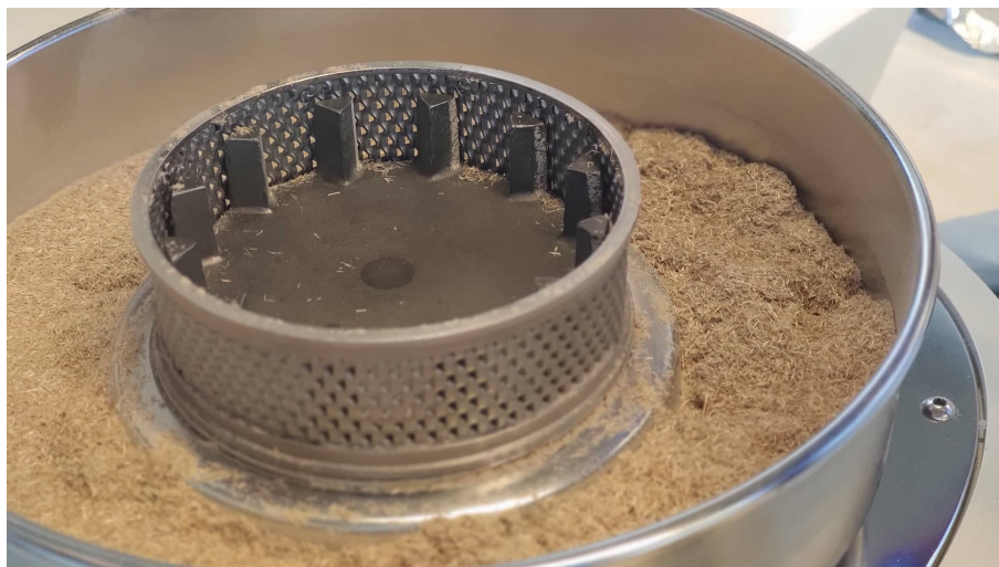
Figure 4.1 Banana fibers in the collecting part of the crushing machine.
