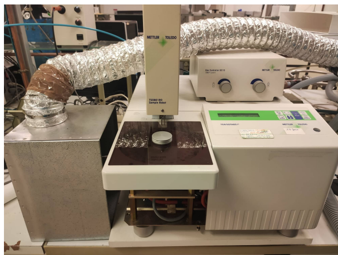
Figure 2.20 TGA/SDTA854e supplied by Mettler Toledo. Device used for laboratory characterisation.
