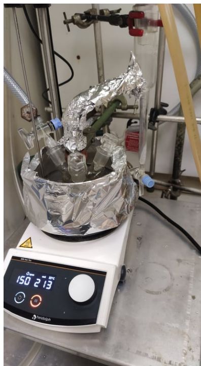
Figure 4.4 Repolymerisation setup under a flux of nitrogen gas and a system of water condensation mixture beside.
