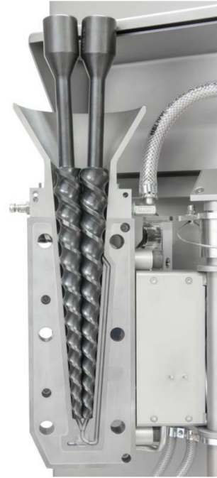
Figure 2.6 DSM - Xplore conical twin-screw extruder. Equiped of a recirculating valve which allows to vary the residence time in the DSM [60].
