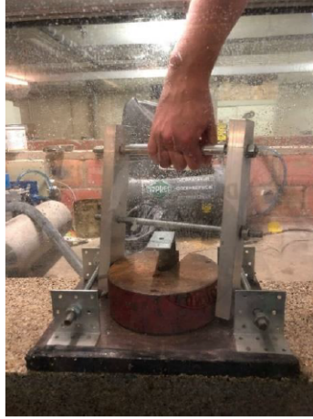
Figure 3.4: The handmade system that permit to compact the sand. Reference: Ilaria Fent's thesis, 2018 [9].
