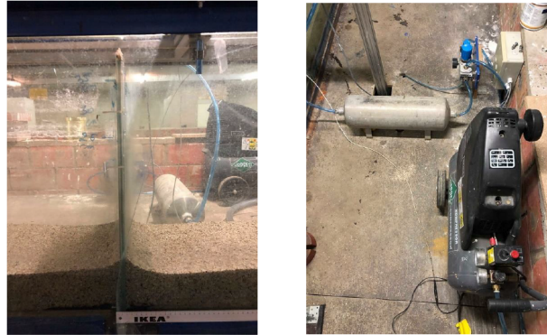
Figure 3.3: On the left: The door that simulates the dam. On the right : The compressor.
