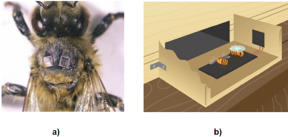
Figure 2.8: RFID technology. (a) Bee equipped with tag from [16] (b) Principle schematic from [36]
