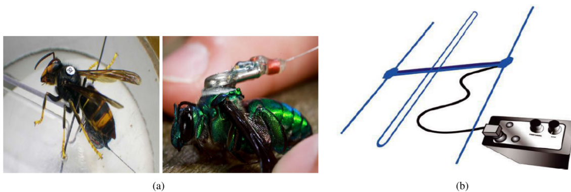
Figure 2.13: Examples of radio telemetry tracking. (a) Asian hornet and bee with transmitters (b) receiver and Yagi antenna from [16]
