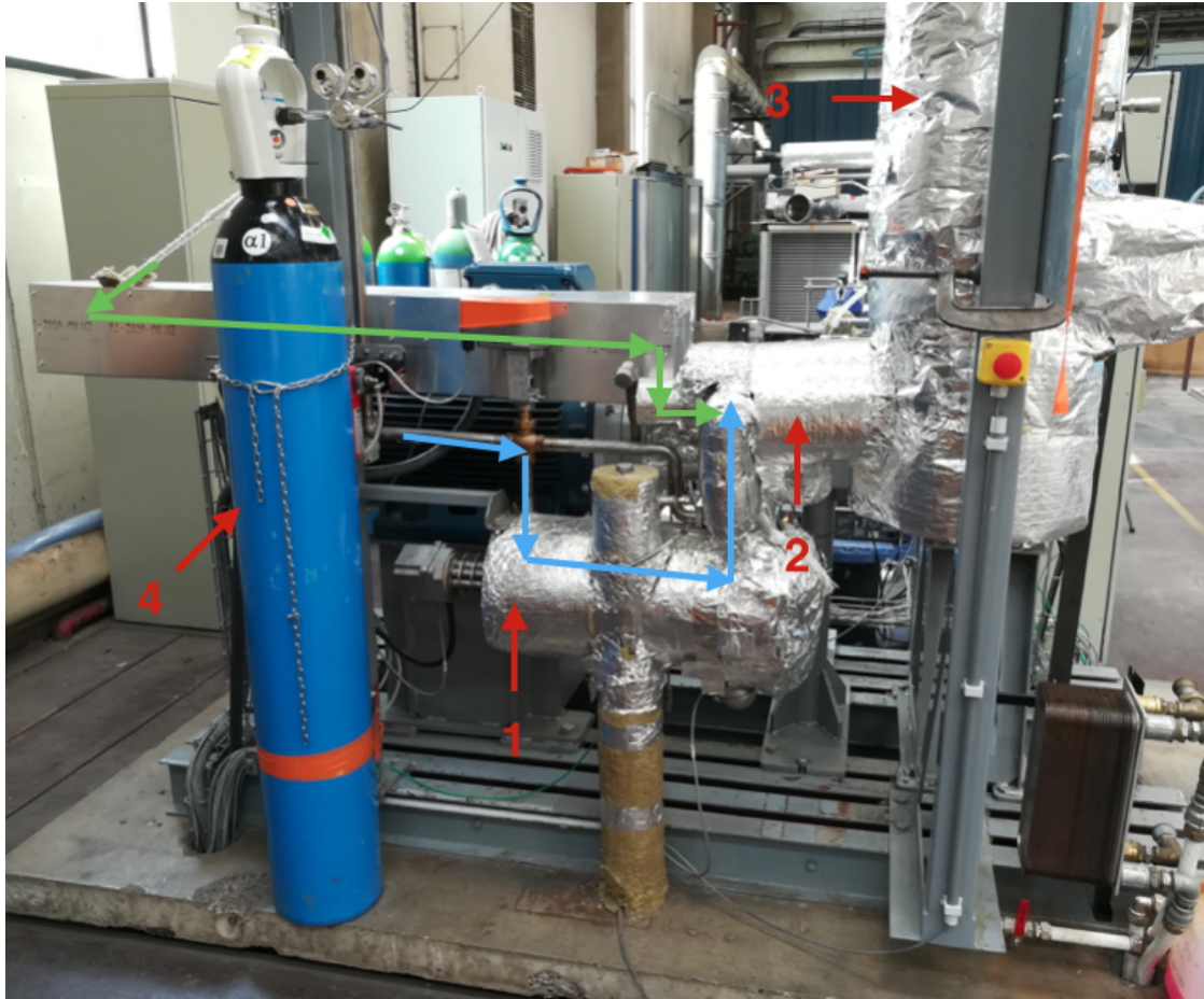
FIGURE 2.10: HCCI test bench, view from the intake side : (1) electric heater, (2) gas mixer, (3) surge drum, (4) nitrogen bottle, green arrows represent the hydrogen flow, blue arrows represent the air flow.
