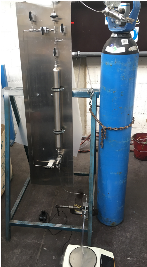
(A) Setup used for the calibration measurements.
