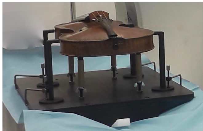
Figure 3.11: Support created to carefully calibrate the positioning of the violin
