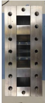
Figure 3.13: Inlet of the nozzle.
