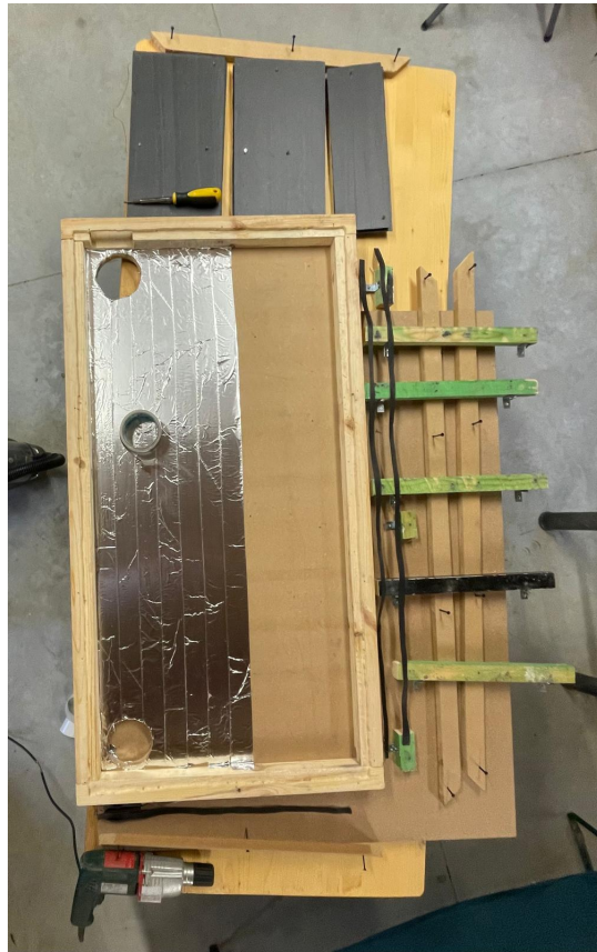
Figure 2.14: Adding of the aluminium foil
