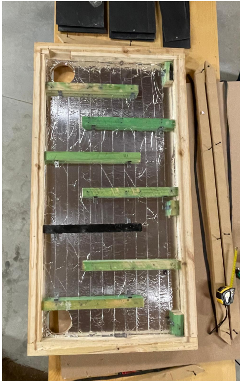
Figure 2.17: Change from 5 to 7 baffles
