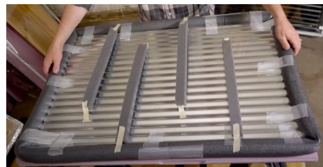
Figure 1.2: Baffles of the DIY collector from NightHawkIngLigth
