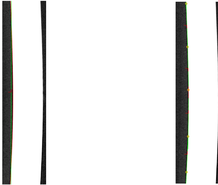
(a) 2D roughness computation using a single linear baseline (code 1). (b) 2D roughness computation using multiple linear baselines (code 2).
