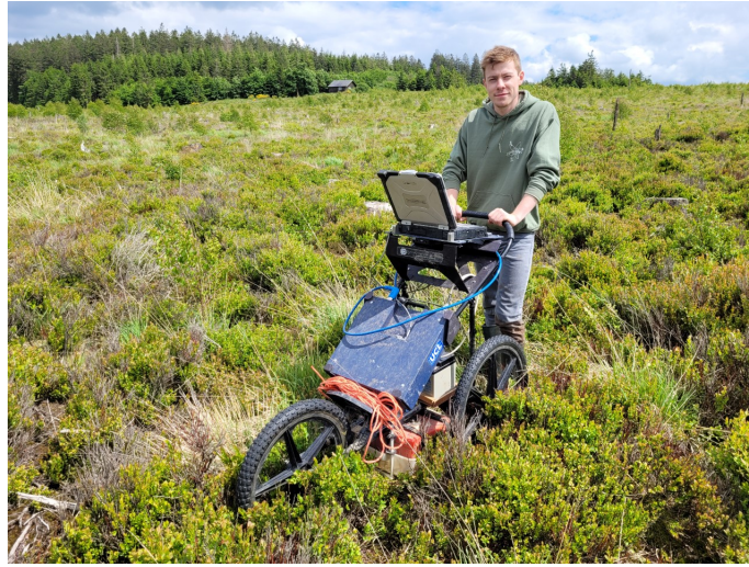
Figure 17: GPR system used during the measurements from June 1 st 2022. Picture taken by Pr. Lambot Sébastien
