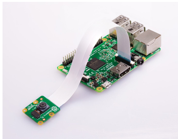
Figure 1.9: Raspberry pi + camera
