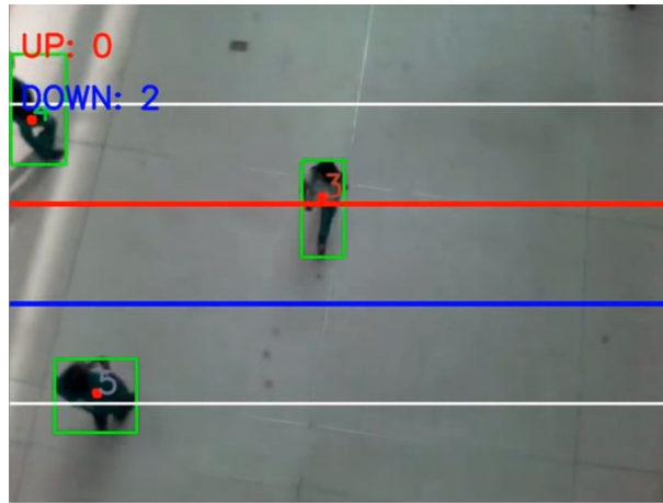
Figure 1.7: Example of motion detection application
