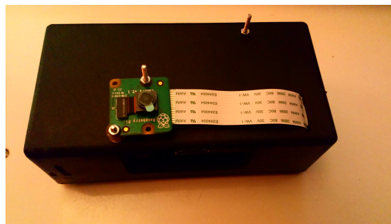
Figure 1.10: Raspberry pi + camera inside a home-made case. That case can then be placed on the ceiling using Double-sided tape for simplicity
