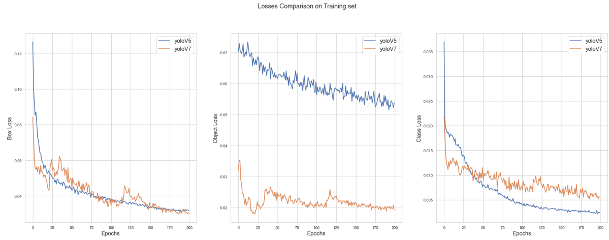
Figure 5.4: YOLOv5 & YOLOv7 results training set
