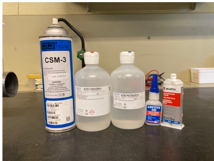
Figure 7.10: Chemicals used for surface preparation
