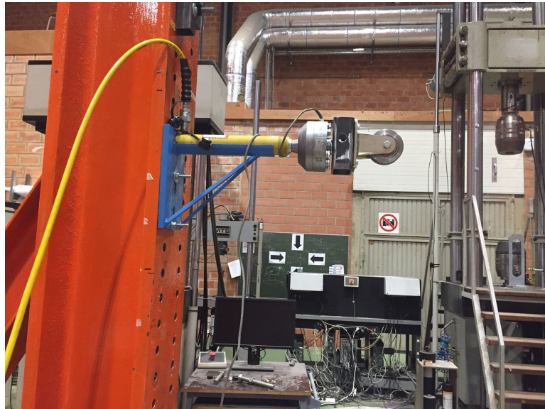
Figure 7.15: Real lateral loading device
