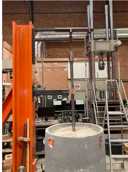
Figure 7.20: Position of rod guide, hammer and anvil
