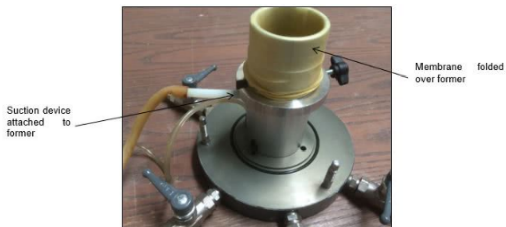
Figure 4.12: Suction device to apply vacuum between the mould and the membrane [66]
