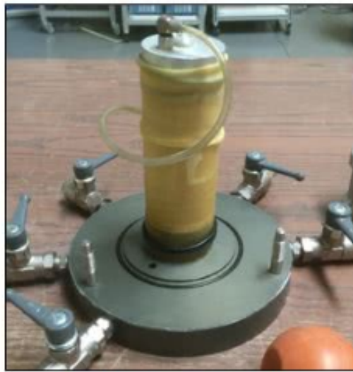
Figure 4.13: Preparation of the sand sample [66]
