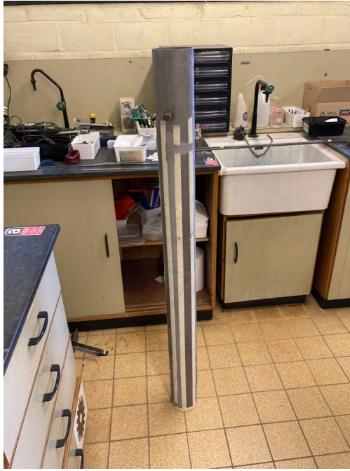
Figure 7.8: Pile taped around the future fibre course
