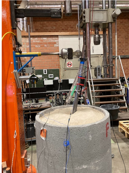
Figure 7.24: Position of the pile after the second lateral loading
