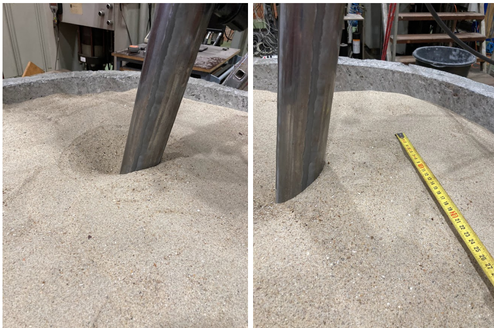
Figure 7.25: Measurement of the sand displacement during the lateral loading
