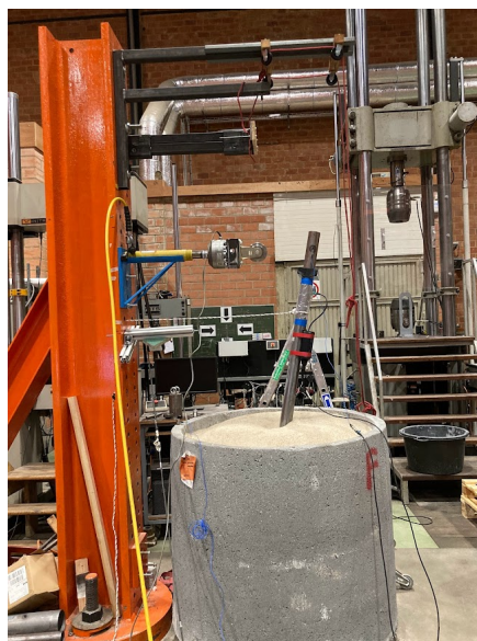
Figure 7.23: Position of the pile after the first lateral loading
