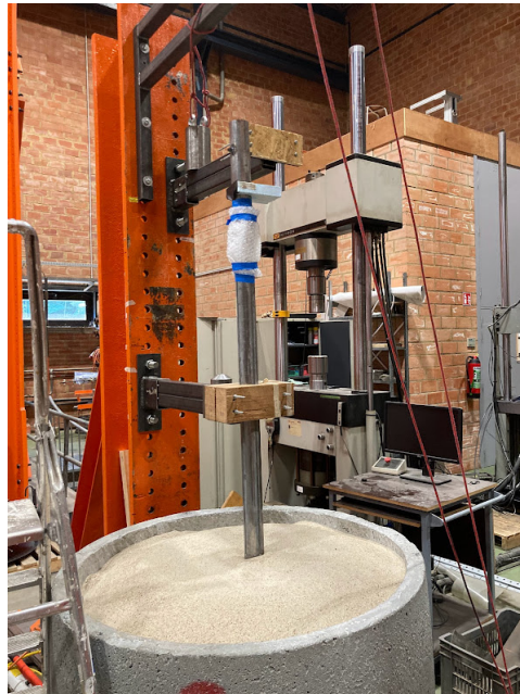
Figure 7.19: Position of pile in the tank
