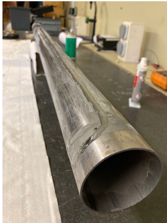
Figure 7.13: Fibre glued on the pile
