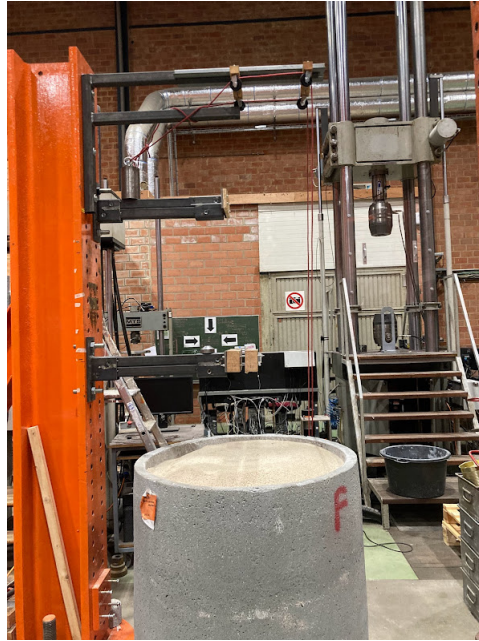
Figure 7.18: Position of lateral guide supports and hammer on the H-column
