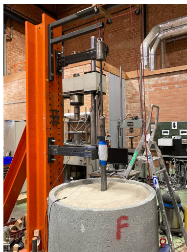
Figure 7.21: Position of the pile at the desired driving depth
