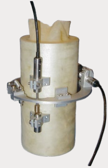
Fig. 2 LVDT transducers as shown on sample.
