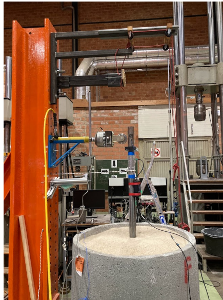
Figure 7.22: Position of lateral loading device, optical fiber device and laser
