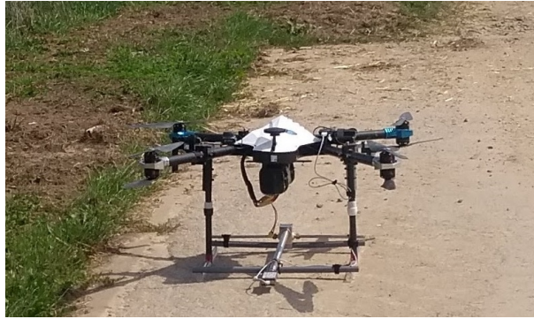
Figure 5.2: Drone-borne ground penetrating radar setup.
