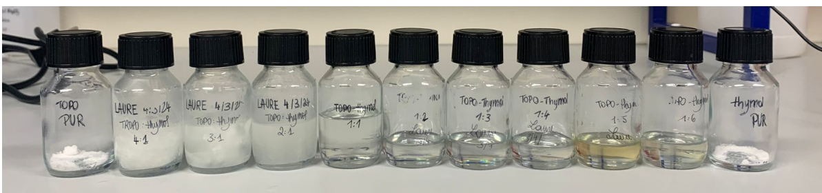
Figure 3.7: Prepared DES mixtures with TOPO and thymol varying molar ratios. Thymol molar ratio increasing from left to right.
