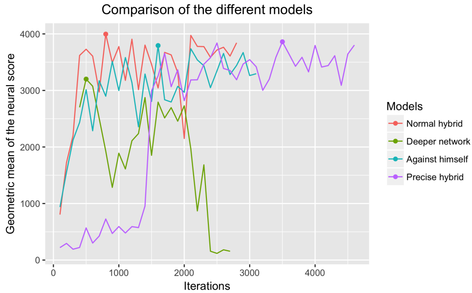
Figure 5.21: The convolutional-LSTM hybrid architecture was omitted because of its poor performances and short training. The y axis is the geometric mean of the neural score over the five sample bots. The dots correspond the the best iteration for each model.
