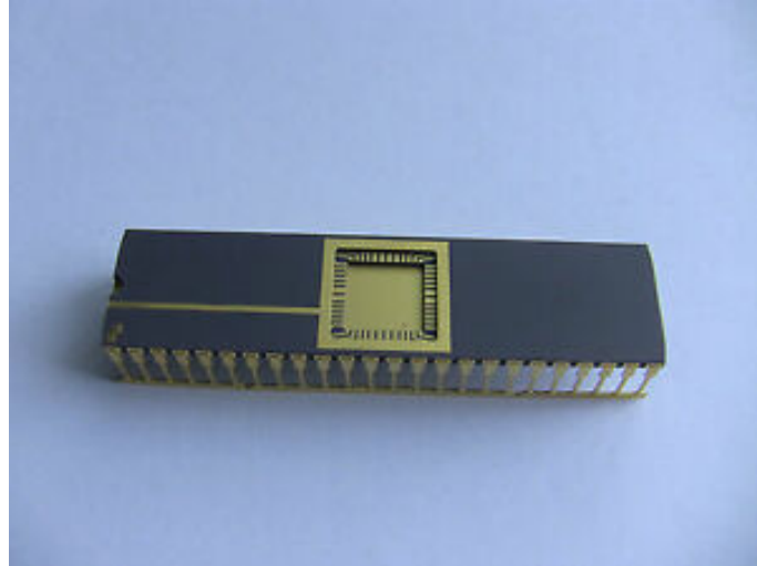
Figure 4.29: Specimen holder constituted of 40 small metallic pins connected to 40 larger ones.
