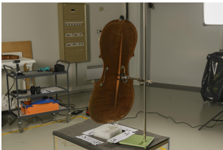
FIG. 3.6 – Setup for the photogrammetry at the Musée de la Musique in Paris, sound board of instrument inv. no. 2020
