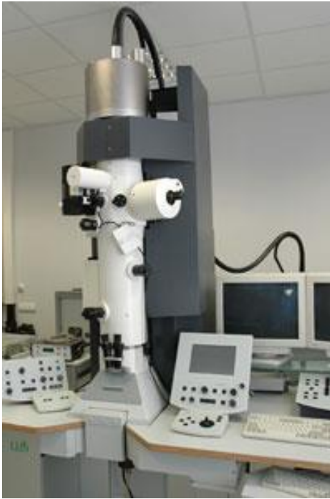
Figure 3.8 LEO 922 TEM microscope, left, and the schematics of different parts of TEM structure, right. [92, 93]
