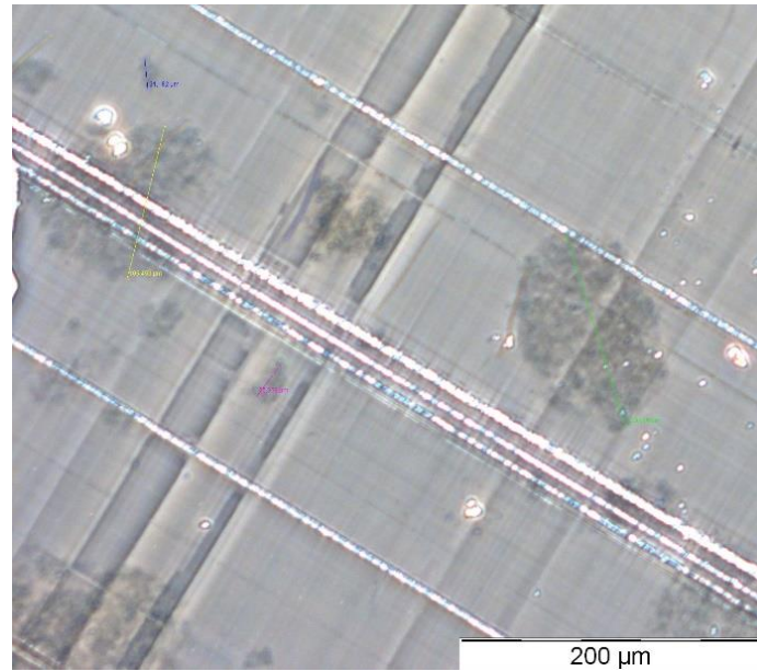
Figure 4.6 Optical microscopy image of sample with 1.0 wt% CNTs
