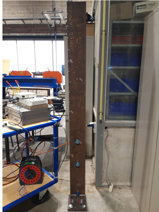
Figure 2.11: Steel plate OMA test setup.
