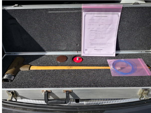
Figure 3.8: Impact hammer used for the experiment.
