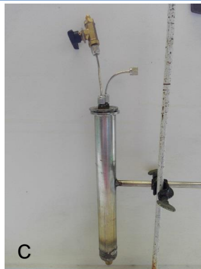
Figure 4-6: (A) Scheme of CO 2 desorption using design C3. Cylindric inox recipient (B) unassembled and (C) assembled.
