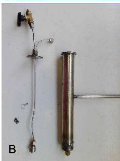
Figure 4-6: (A) Scheme of CO 2 desorption using design C3. Cylindric inox recipient (B) unassembled and (C) assembled.
