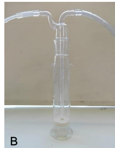
Figure 4-5: (A) Scheme of CO 2 desorption using immersed resin, design C2. (B) Close-up of the glass recipient with the dipping tube and resins in suspension.
