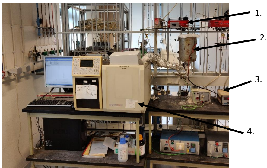
Figure 2.1: Photography of the catalytic setup used during this study. 1. Syringe pump, ethanol inlet. 2. Reactor. 3. Gas flow controller for H_2 and N_2 . 4. Gas chromatograph.
