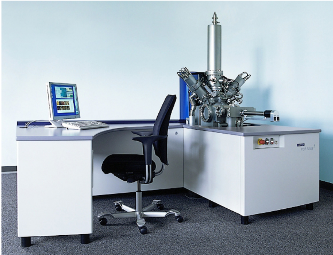
Figure 1.11: An IONTOF V system, similar to the one used for this work (from www.iontofs.com )
