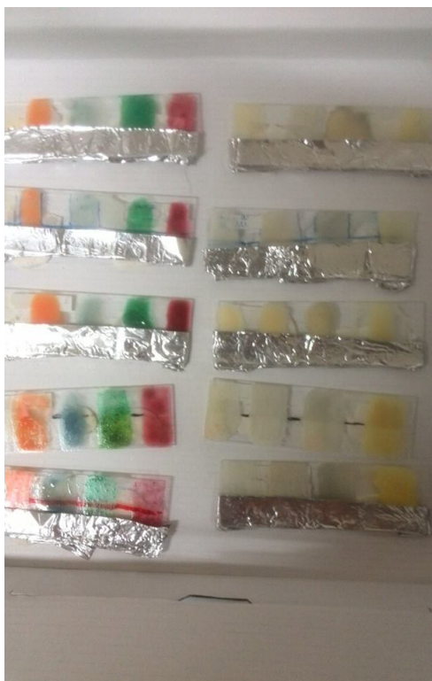
Figure 1.3: One complete series of glass plates. Four such series were made (three on glass plates and one on cardboard). Eight of the ten plates are visible with the aluminium foil covering one half.
