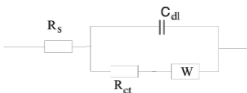
Figure 4.14: Randle circuit with added Warburg element to model the ion diffusion from the bulk solution to the electrode surface [99].
