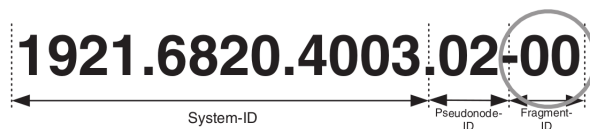
Figure 4.1: The LSP-ID one byte dedicated to fragmentation.
