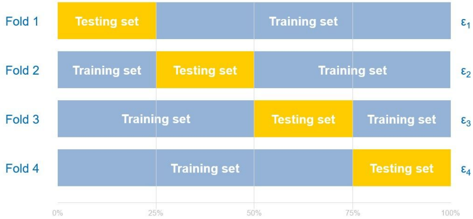
Figure 5.1: Illustration of cross-validation with 4 folds. Reproduced from [52].
