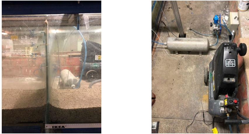
Figure 3.4: On the left: View of the canal gate - On the right: Pneumatic system Reference: Donifan Camacho-Fernandes and Pauline Radelet's Master thesis (2019)
