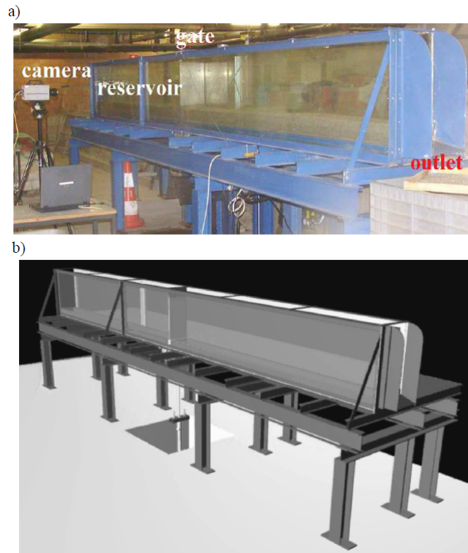
Figure 3.1: Dam break channel in the Hydraulic Laboratory of UCLouvain. a) photo at the laboratory; b) overall view from Spinewine (2005) Reference : Ilaria Fent's thesis (2018)
