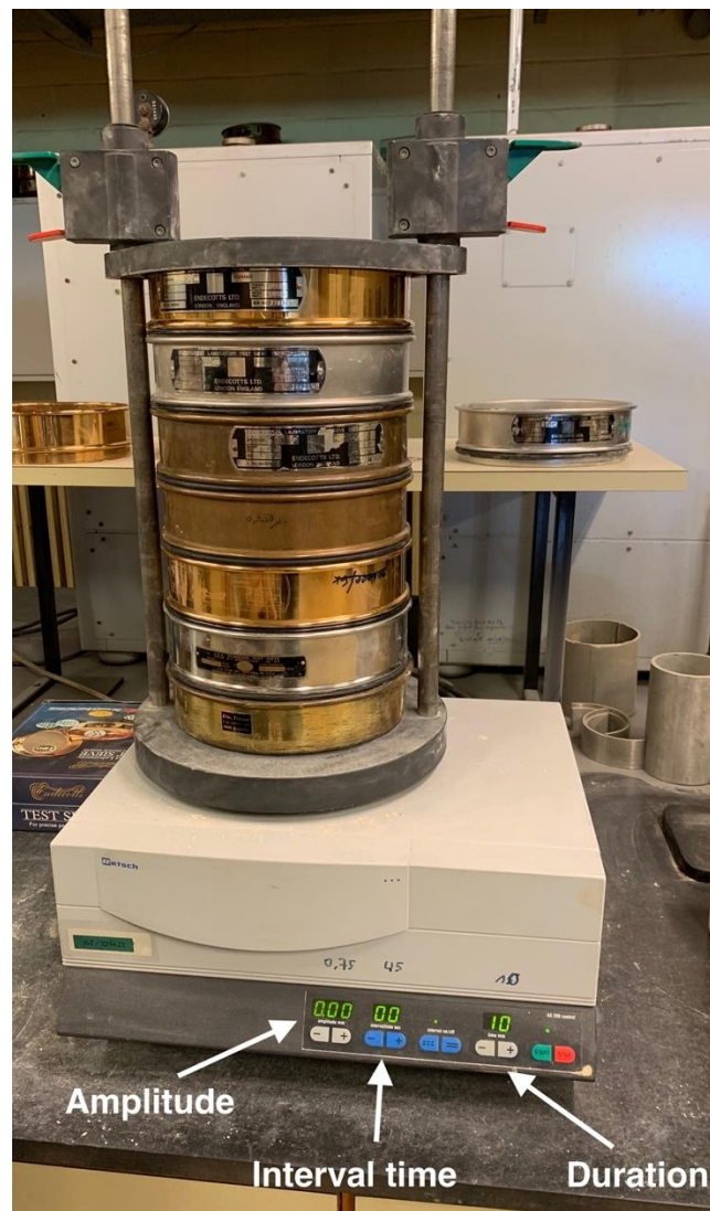
Figure A-1: The tephra was dry sieved during 10 minutes using an AS 200 Control Retsh vibrating sieve shaker with six sieves (63; 125; 250; 500; 1,000; 2,000 \mu\text{m} ). The amplitude was set at 1.23, the interval time at 2 seconds and the duration at 10 minutes.
