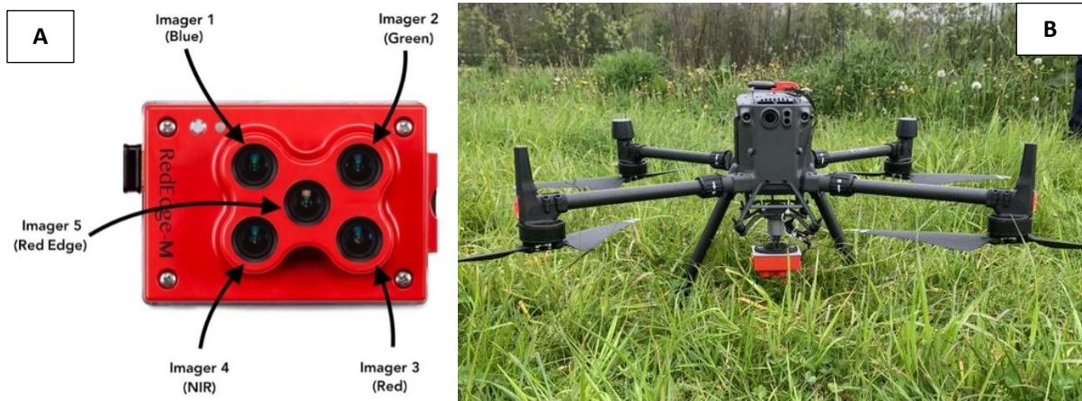
Figure 22: MicaSense RedEdge-M multispectral camera, with the five imagers recording the different spectral bands (A). Source: MicaSense, 2017. Drone DJI “Martice 300 RTK” with the MicaSense RedEdge-M mounted on it (B).
