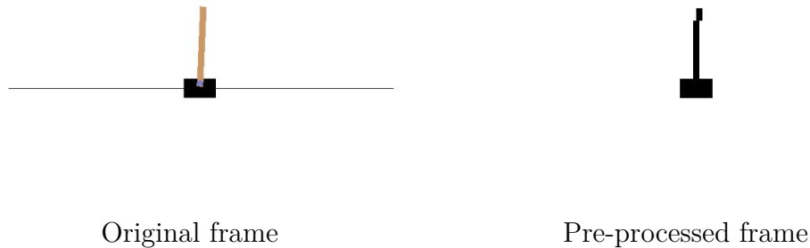
Figure 4.1: On the left, the frame produced by the gym environment. On the right, the image pre-processed which is given to the agent to learn.
