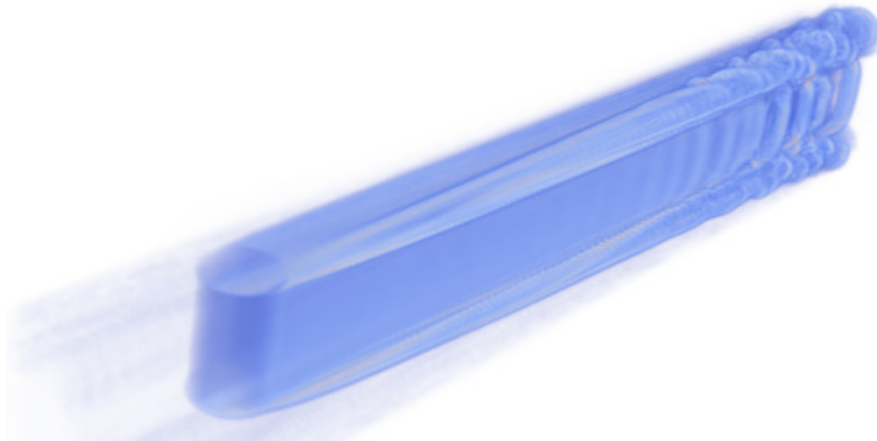
Figure 4.19: Volume rendering of the vorticity magnitude in the wake of the ACM for TSR 2.14.
