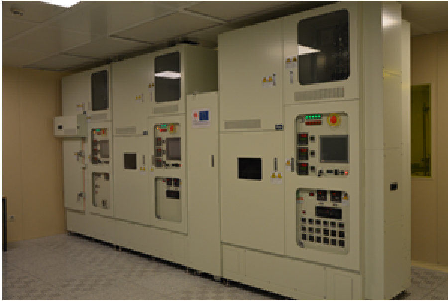
Figure 3.2: Koyo vertical furnace. It can hold 25 wafers of 3 inches.
