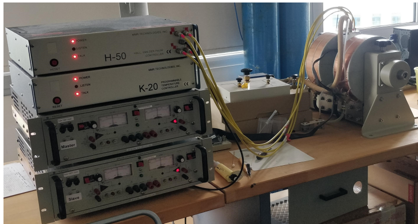
Figure 3.51: Photo of the hall setup. The electromagnet is on the right and the different SMU and temperature controller are on the left.
