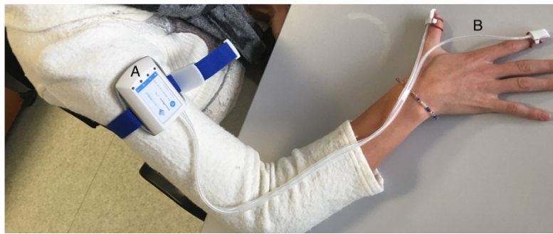
Figure 1.1: Bluetooth module (A) attached around the arm using provided strap; Finger sensors (B) attached around the fingers using silicon rubber bands
