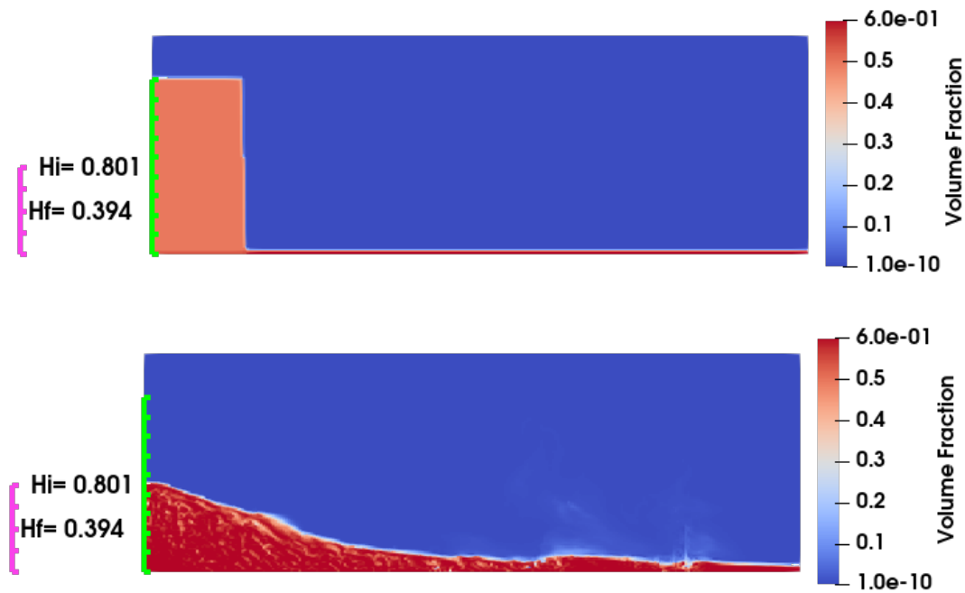
Figure 6.2: Simulation results (Initial and final situation) from the model and algorithm of Chapter 2 for aspect ratio A=2 , initial volumetric fraction of 0.495 and parameters of sand used in laboratory.
