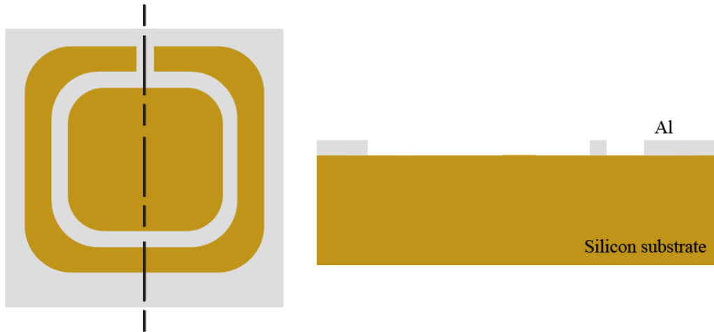
Figure 3.13: Schematic diagram showing (a) top view and (b) cross-sectional view of the silicon substrate after aluminum metallization and lift off.
