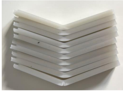
Figure 47 Injected PLA/rPMMA bars tested
