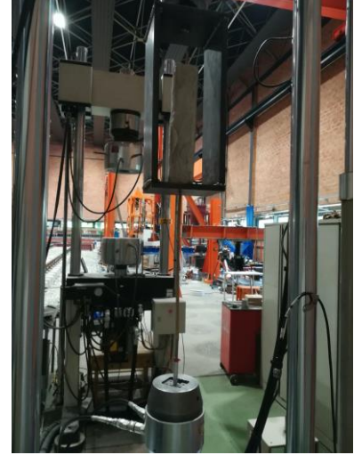
Figure 57 Pull-Off test device at LEMSC
