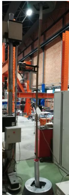
Figure 53 Traction test device at LEMSC
