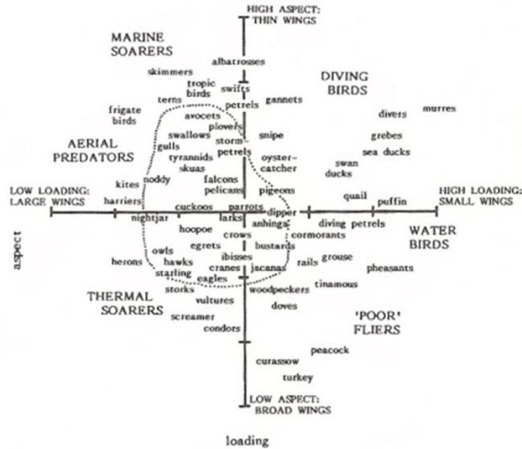
Figure 5.1 – Wing loading versus Aspect ratio. The ibises appear on the schematic to be average flyers. They are quite close to egrets and cranes and less from herons and pelicans. (Figure taken from http://people.eku.edu/ritchisong/554notes2.html )
