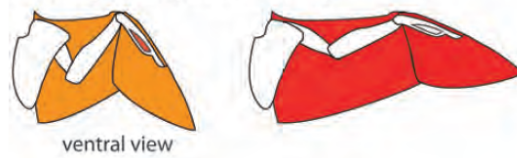
(a) Wing folding or expanding - 3 rotation DOF constrained kinematically by 2 Equations to achieve 1 movement
