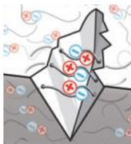
Fig1.5- Self-assembly mechanism by ionic interactions allowing the reversible network.[6]
