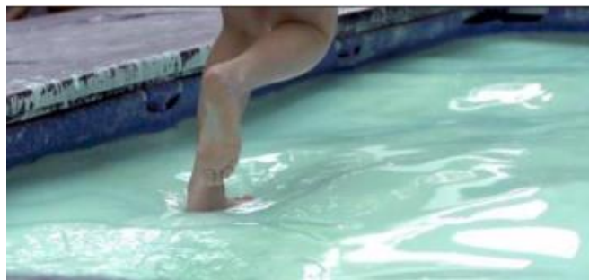
Figure 1.21- Non-Newtonian fluid illustrating the dynamic behavior concept and the Deborah relationship. This cornstarch pool has an interesting behavior, depending on the experimental time. Quickly loaded, it reacts as a solid and slowly loaded, it behaves as a liquid.[6]
