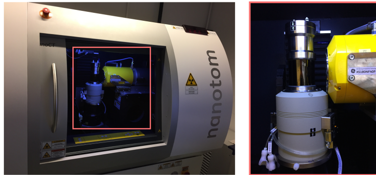
Figure 5.2: Tensile loading stage: Deben MICROTTEST - CT5000-TEC [16].
