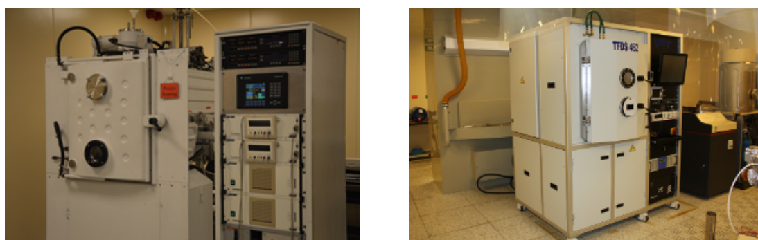
Figure 3.12: The VACOTEC Dual E-gun evaporation system (left) and the VST - TFDS 462 (right) in Winfab at UCLouvain, both used for the deposition of aluminium electrodes (thickness 1\ \mu\text{m} ) on nitrocellulose [202]
