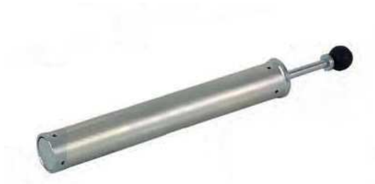
FIGURE 3.3 – Dame de compactage de l'essai Proctor [27]
