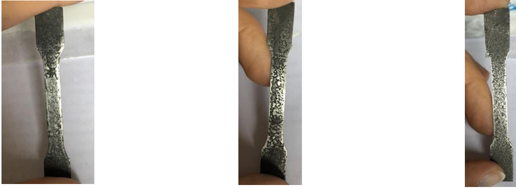
Figure 2.11: State of the surface of the Specimen 0h , the Specimen 8h and the Specimen 24h (from right to left)
