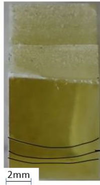
Figure 5.17: Fracture surface of sample SENBAmb.6 with some lines indicating some jumps of the propagating crack are observed.
